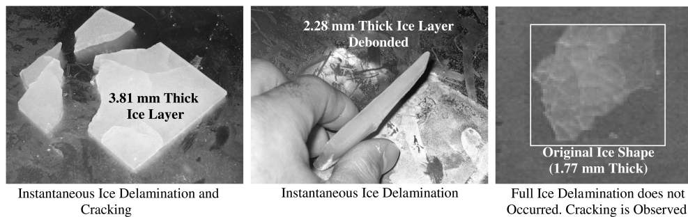
Fig. 12 Experimental ice debonding and fracture patterns under ultrasonic ZX and XY shear stresses (28.5 kHz, 50 V, -20^{\circ}\text{C} ). Patterns agree with finite element method predictions.
